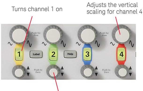
Vertically positions the waveform on channel 2
