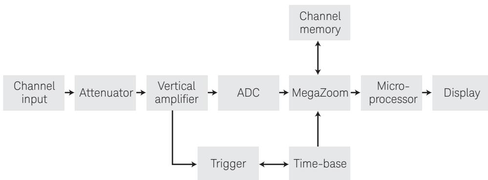
Figure 12. Digitizing oscilloscope architecture.
