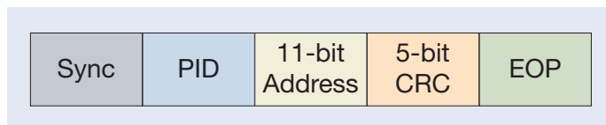
Figure 19. OUT, IN and SETUP token packet organization.
