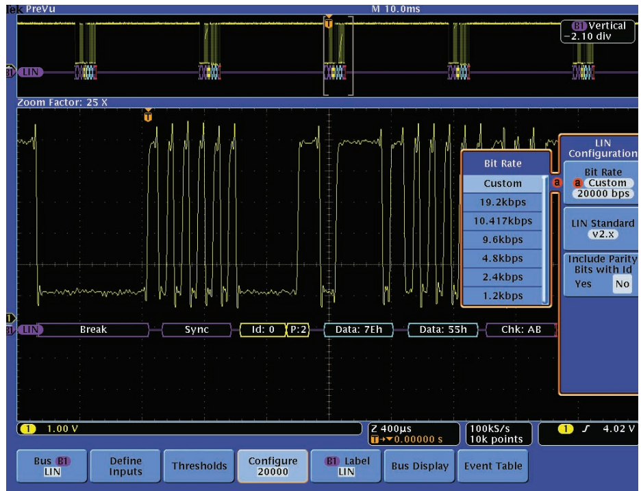
Figure 31. LIN bus setup menu and decoded frame.
