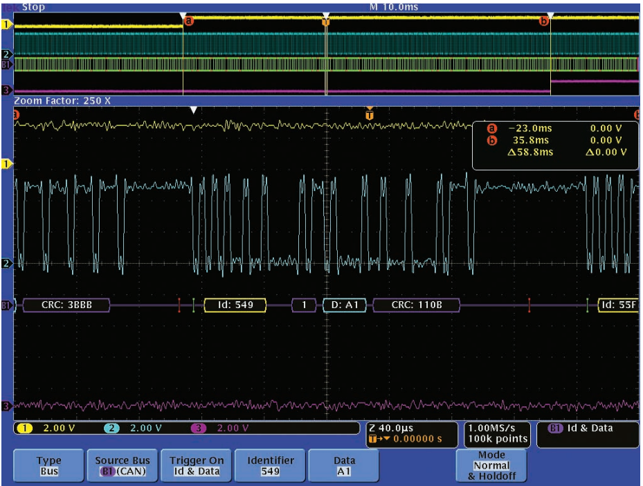
Figure 28. Triggering on specific identifier and Data on a CAN bus and decoding all messages in the acquisition.
