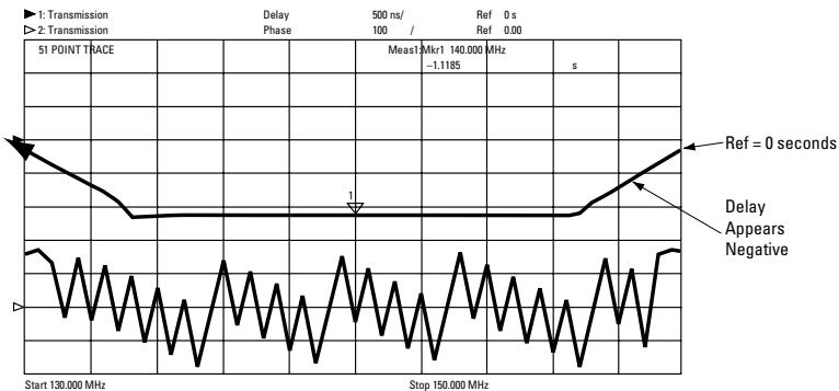
Figure 9. Filter measurement with insufficient number of points
