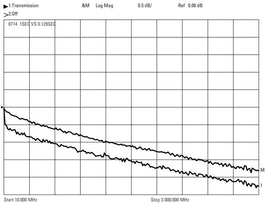
**Figure 4.** Reduce measurement error by increasing swap time
