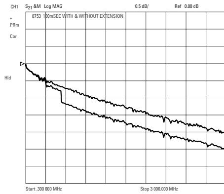
**Figure 5.** Reduce measurement error by balancing reference path
