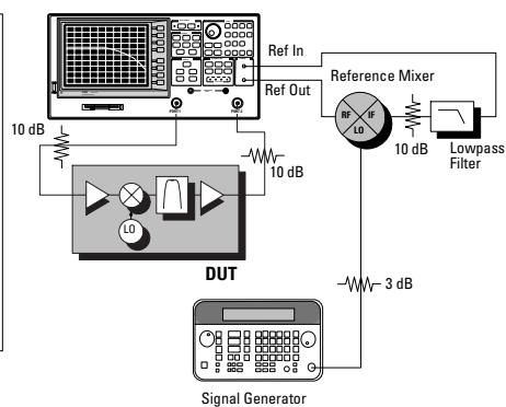
**Figure 7B.** High dynamic range conversion loss measurement (left) and high dynamic range setup (right)
