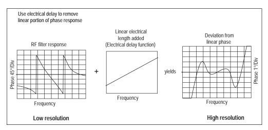
Figure 12: Deviation from linear phase
