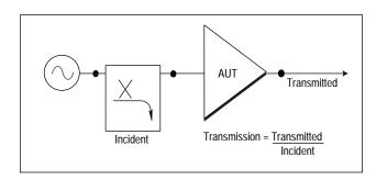
Figure 10: Network analysis transmission measurements
