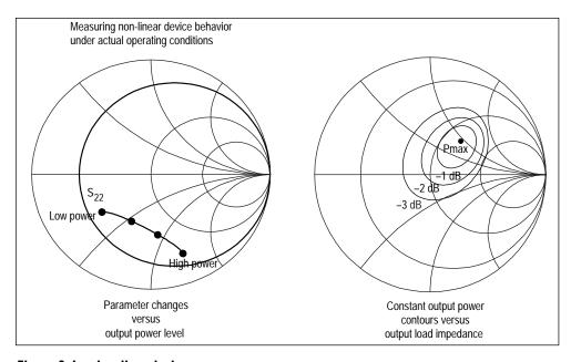
Figure 9: Load-pull analysis
