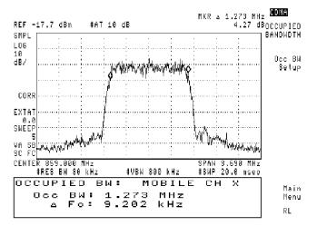
Figure 22: Occupied bandwidth measurement
