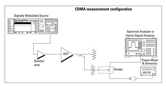
Figure 7: Test configuration for in- and out-of-channel measurements
