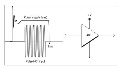
Figure 8: Pulsed-RF network analysis
