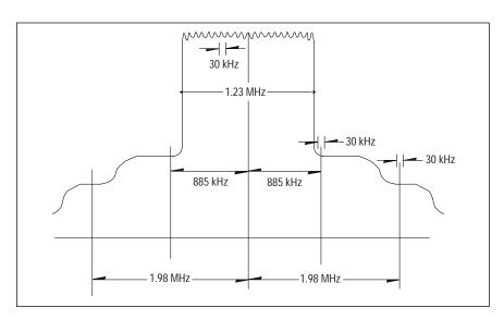
Figure 24: Example ACPR specification
