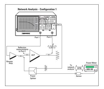
Figure 5: Network analysis configuration for forwarddirection measurements
