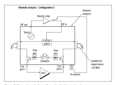
Figure 6: Network analysis configuration for forward and reverse measurements
