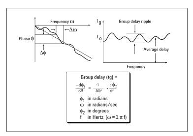
Figure 13: Group delay calculation
