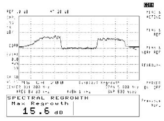
Figure 28: Spectral-regrowth measurement
