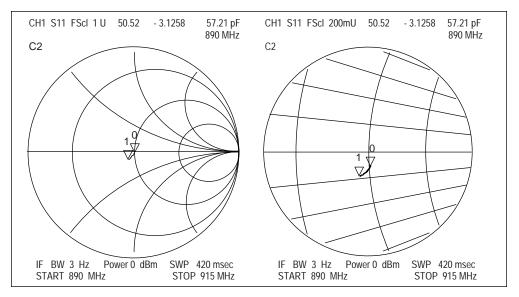
Figure 18: Input impedance measurement
