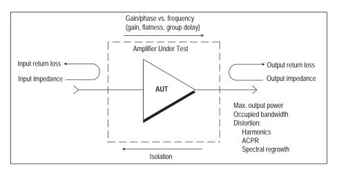
Figure 1: Common amplifier measurements
