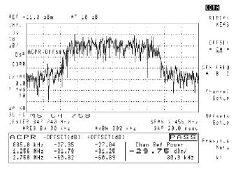
Figure 26: Adjacent-channel-power-ratio measurement
