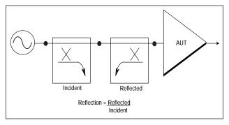
Figure 16: Network analysis reflection measurements
