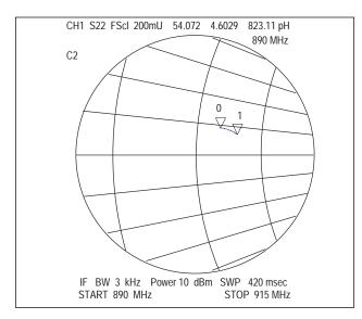
Figure 19: Output impedance measurement
