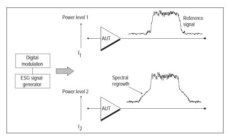
Figure 27: Intermodulation distortion causes spectral regrowth
