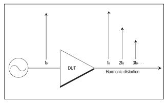
Figure 23: Harmonic distortion caused by non-linearities in the amplifier
