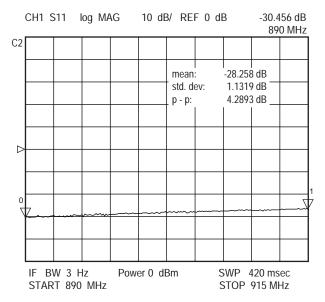
Figure 17: Return loss measurement
