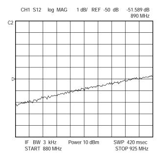
Figure 15: Reverse isolation measurement
