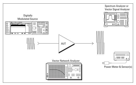
Figure 4: Test instruments for making stimulus response measurements
