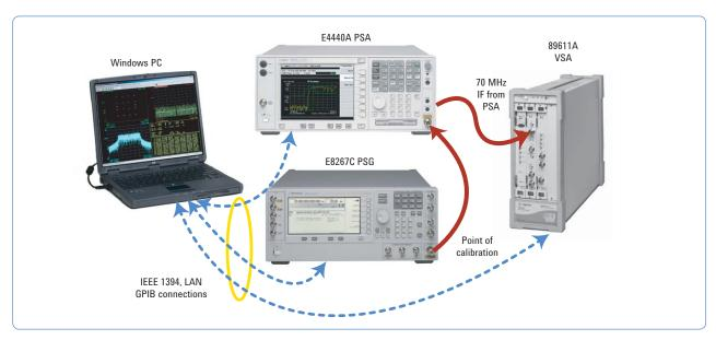
Figure 2. 89611A VSA with PSA (70 MHz IF out) calibration system, equipment setup example
