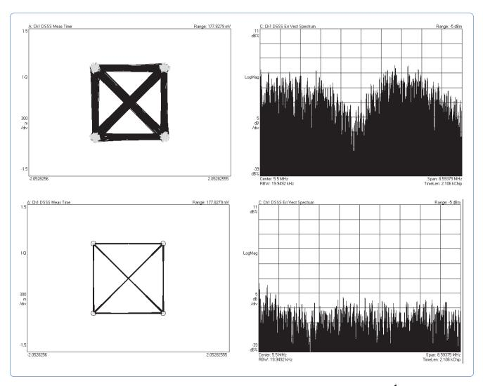
Figure 13. 802.11b error vector spectrum and constellation before (top) and after (bottom) extended calibration<sup>1</sup>
