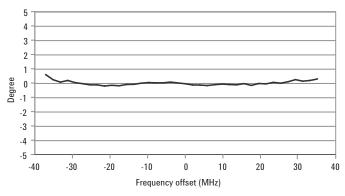
Figure 7. Phase deviation after calibration, 72 MHz span at 18.1 GHz (preselector bypassed)
