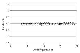
Figure 5. Nominal peak positive and negative amplitude deviation after calibration (preselector bypassed, 64 MHz bandwidth)
