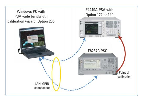
Figure 1. PSA Option 122 or 140 calibration system, equipment setup example
