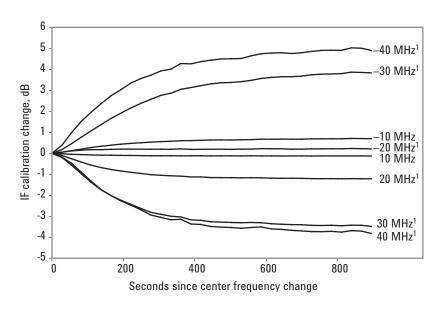
Figure 11. IF calibration change following a 3.1 GHz to 19 GHz center frequency change, for various offsets from center frequency (PSA Option 122)
