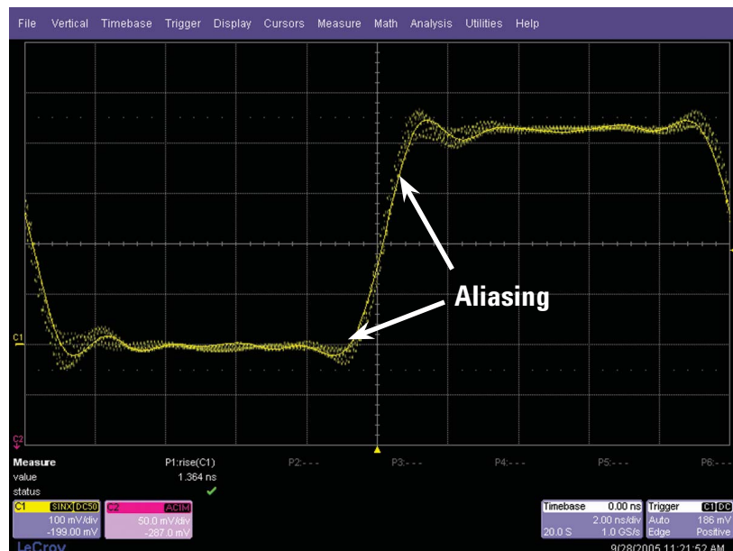
Figure 4: 500-MHz bandwidth scope sampling at 1 GSa/s produces aliased edges
