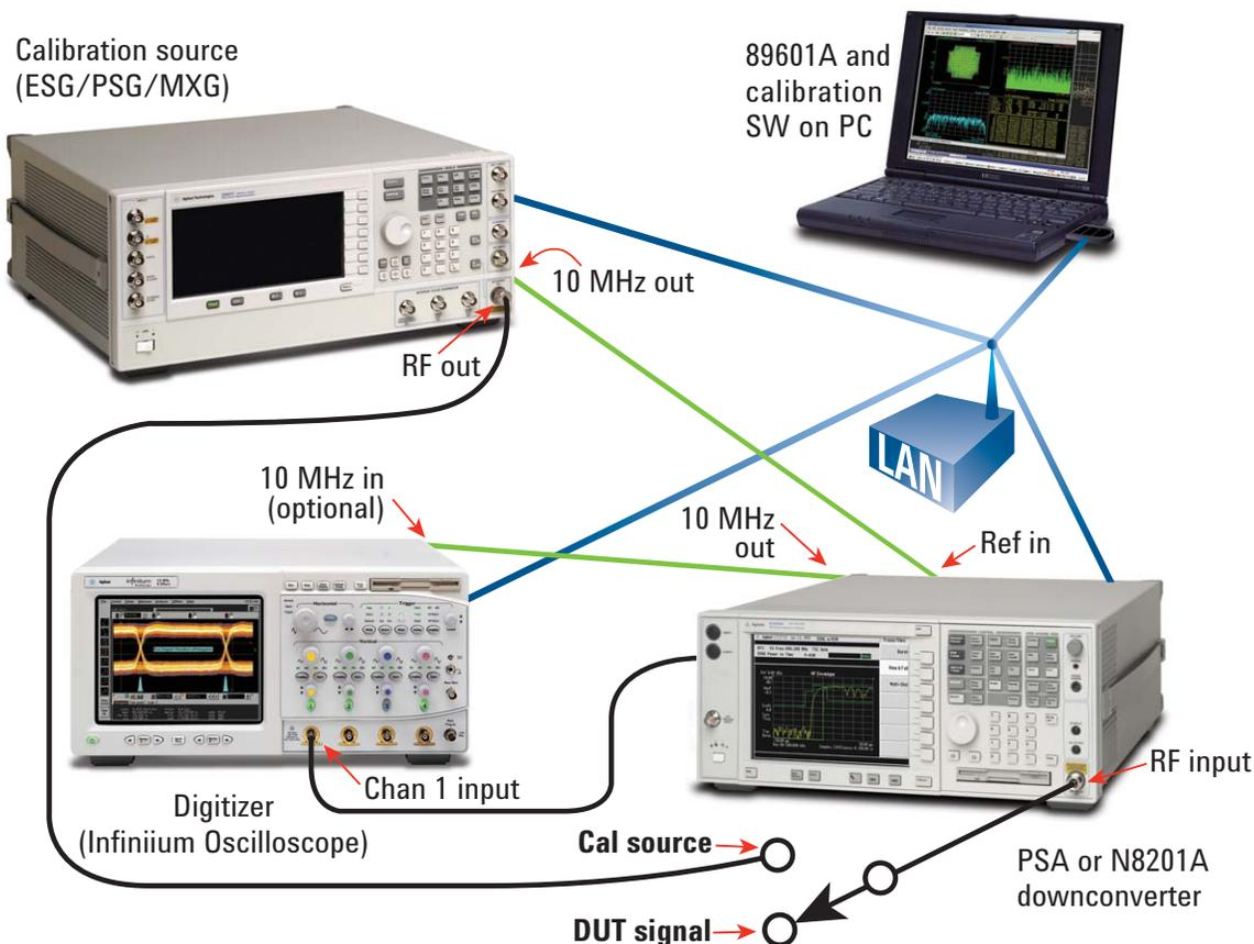
Figure 1. Configuration of VSA software, PSA downconverter, and Infiniium Oscilloscope digitizer.
