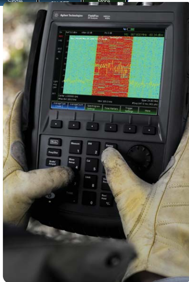
The spectrogram display makes it easy to detect and monitor intermittent interference signals.
