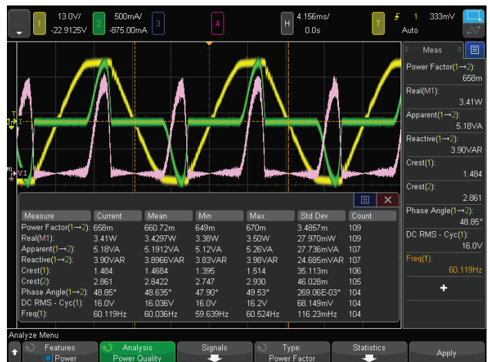
Figure 9: Input Power Quality measurements
