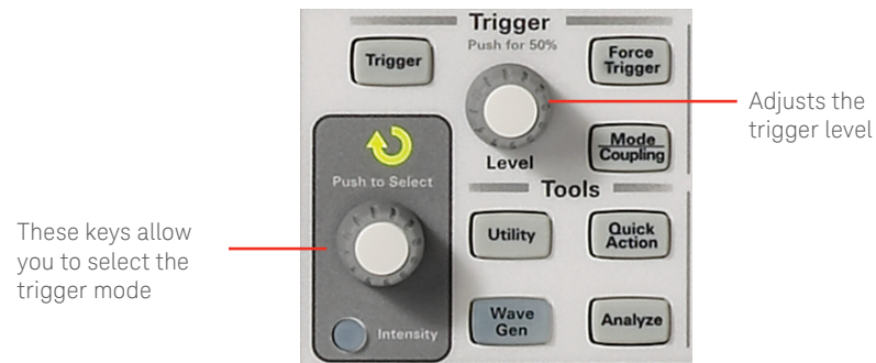
Figure 20. Front panel trigger control section on a Keysight InfiniiVision 2000 X-Series oscilloscope
