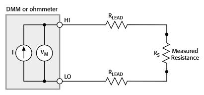
$R_{measured} = R_S + R_{LEAD} + R_{LEAD}$
