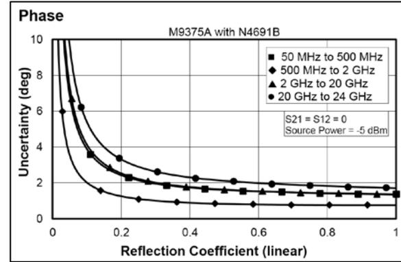
**Table 4. With 85052D standard mechanical 3.5 mm calibration kit <sup>6</sup>**
