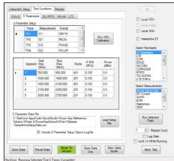
The PXI VNA's multiple programmatic interfaces allow for easy integration into test environments and reduced development time.
