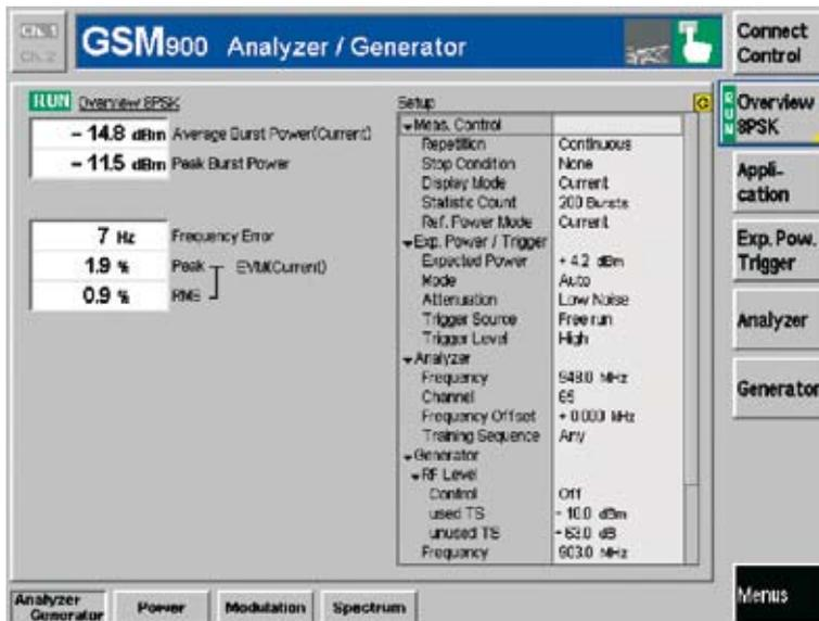
The non-signaling mode allows GMSK/8PSK signals to be generated and analyzed for RX/TX module testing; the hotkeys at the bottom of the screen provide immediate access to specific measurements.
