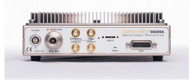
The SM200A is a high-performance spectrum analyzer and monitoring receiver. Tuning from 100 kHz to 20GHz, the analyzer has 160 MHz of instantaneous bandwidth (IBW), 110 dB of dynamic range, 1THz/sec sweep speed at 30kHz RBW (using Nuttall windowing), and phase noise performance that is low enough to contribute less than 0.1% error to EVM measurements and rival even the most expensive spectrum analyzers on the market.
