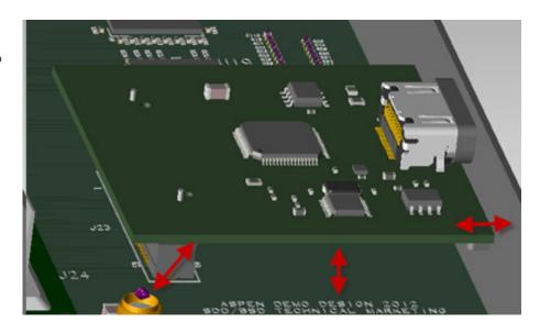
Take measurements in PADS Standard in a full 3D photorealistic view of your PCB assembly to know the exact distance between objects.
