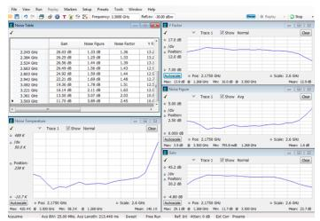
Noise Figure and Gain measurements (Option 14) help you to quickly and easily measure your device using the RTSA and a noise source. This image shows the measurement summary table with graphs of noise temperature, gain, noise figure and Yfactor.
