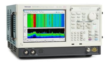
The RSA6000 Series gives you the functionality of a high-performance spectrum analyzer, wideband vector signal analyzer, and the unique trigger-capture-analyze capability of a real-time spectrum analyzer - all in a single package. A typical 20 dBm TOI and -151 dBm/Hz DANL at 2 GHz gives you the dynamic range you expect for challenging spectrum analysis measurements.
