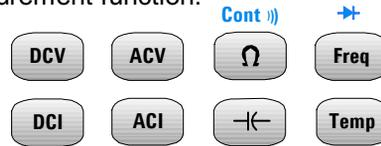
The continuity and diode test functions are shifted (shown in blue). For example, to select continuity, press:
