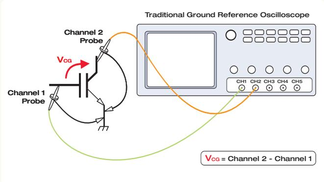
► Example of two probes measuring ground reference voltages.
