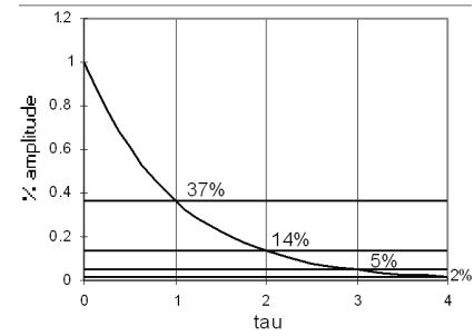
Normal RL or RC time constants are exponential decays. The above shows the remaining amplitude when  $t = \text{time constant } \tau$ .
