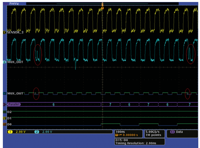
Figure 7. CH2 shows more detail for MUX_OUT.
