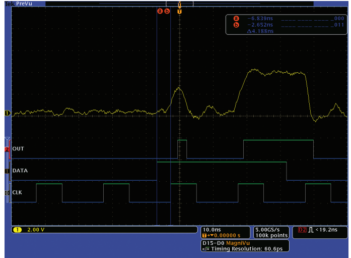
Figure 20. D-Flip-Flop Q output error with analog insight.
