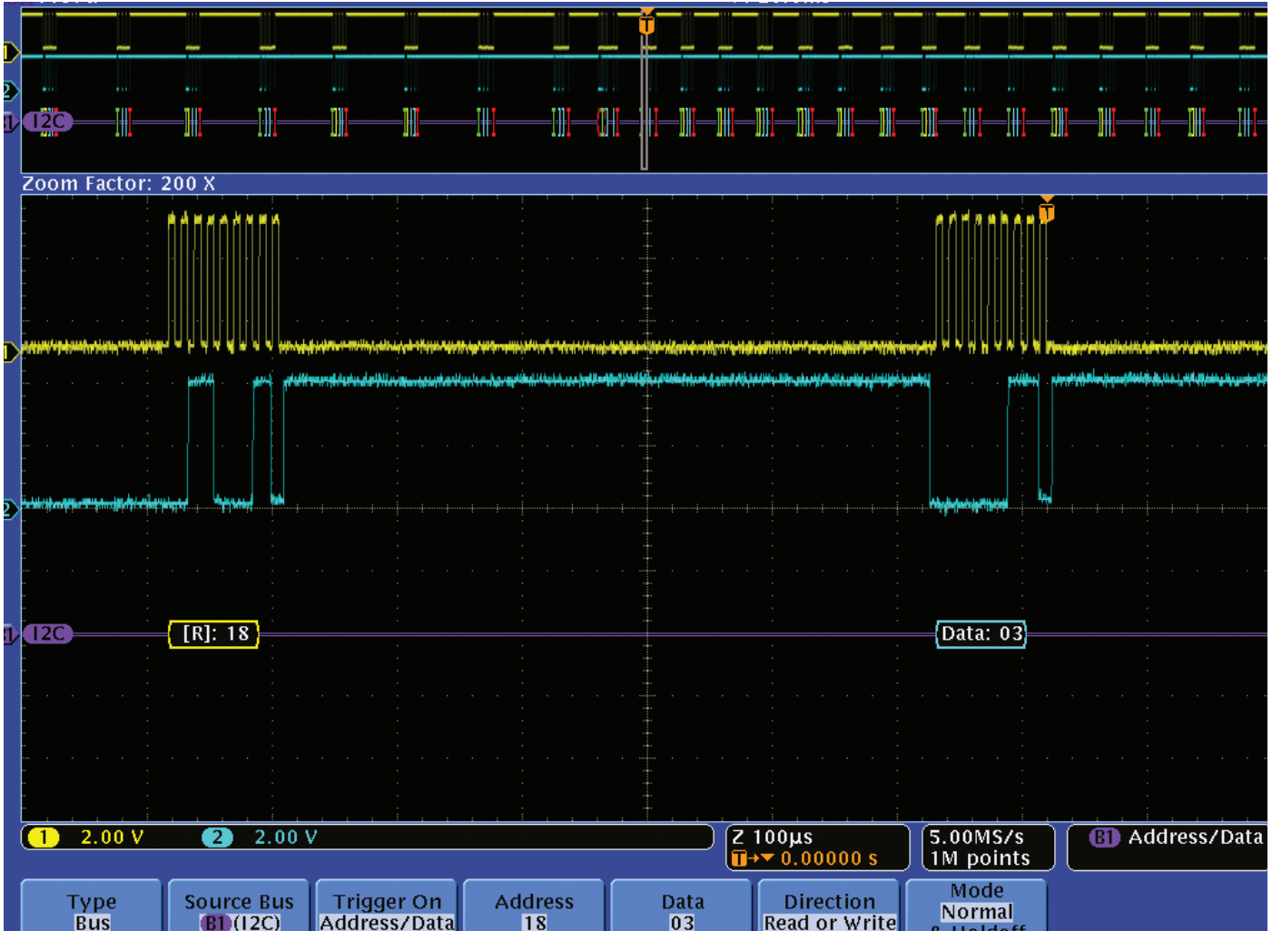
Figure 2. Navigating through a long acquisition of an I2C bus.
