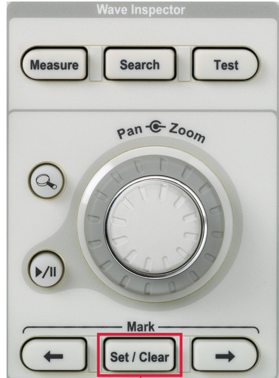
Figure 2B. Dedicated front-panel controls for setting/clearing marks and navigating between them.
