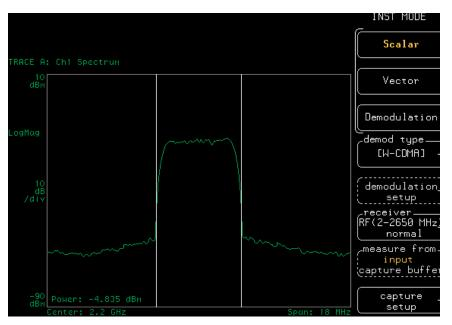
Examine the W-CDMA spectrum and make power measurements using band power markers.
