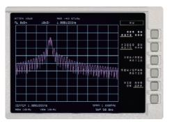
The Agilent 8560 EC-Series provides a complete solution for adjacent channel power (ACP) testing of burst carrier signals using digital modulation as well as the ability to measure occupied bandwidth percentage. Time-gated signal analysis lets you easily measure a wide variety of time-varying signals, such as pulsed RF, time division multiple access (TDMA), interleaving, and burst modulation.
