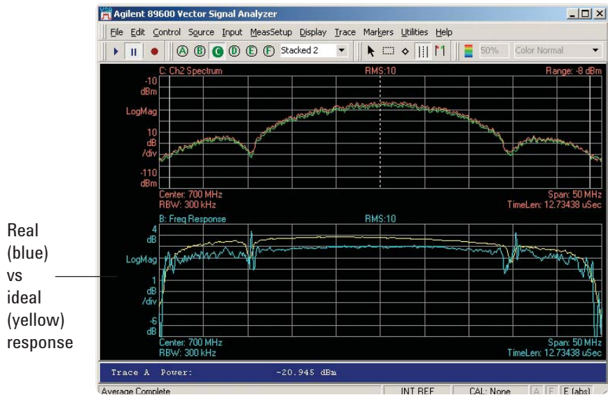
Figure 5. Finding the 1-dB compression point of an amplifier using real-world signal as stimulus.
