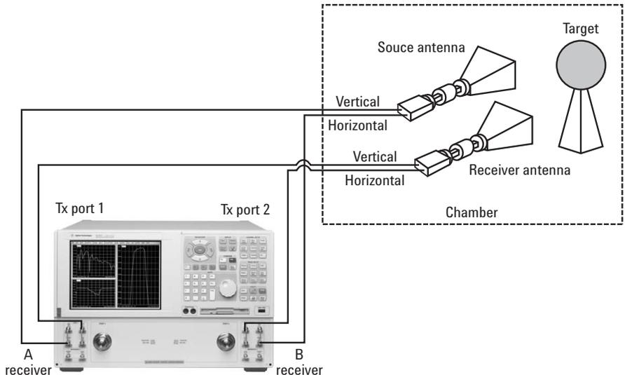
**Figure 2: Typical RCS measurement configuration for measuring the full polarization matrix, using the PNA receiver.**
