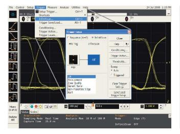
Figure 1. InfiniiScan menu is conveniently located by the trigger menu
