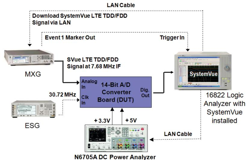
Figure 32. LTE OFDMA SISO BER test setup using connected solutions
