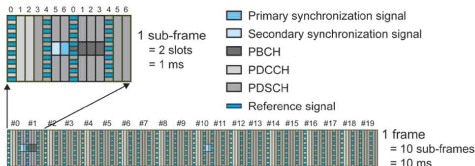
Figure 25. Example of downlink mapping (normal cyclic prefix)
