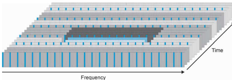
Figure 26. Example of downlink mapping showing frequency (subcarriers) vs. time
