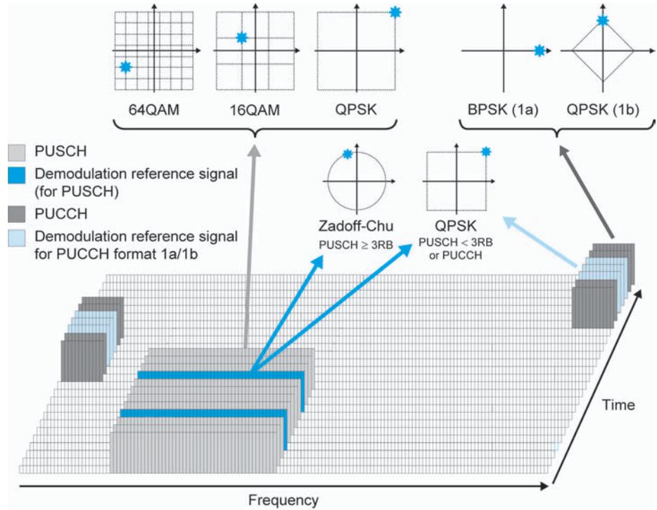
Figure 27. Example of uplink mapping showing frequency (subcarriers) vs. time
