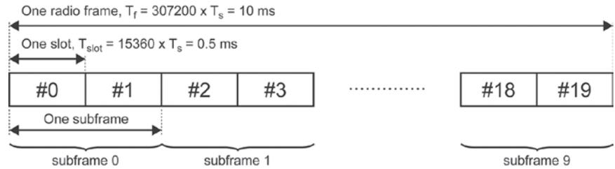
Figure 21. LTE frame structure type 1 (36.211 [10] Figure 4.1-1)
