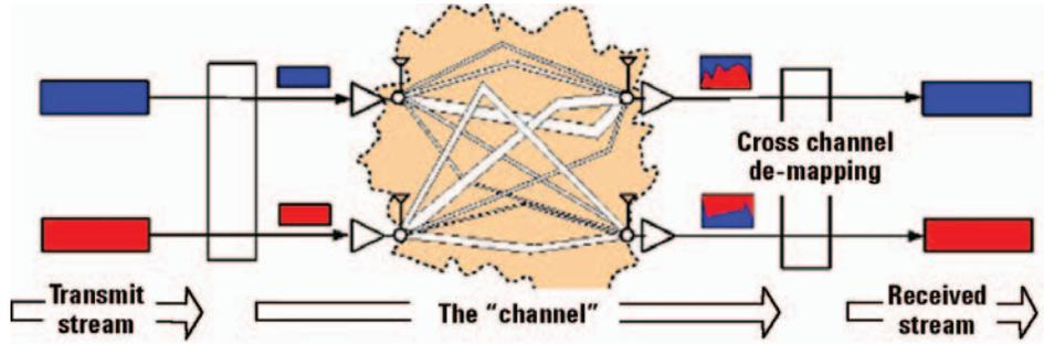
Figure 16. 2x2 MIMO, no precoding
