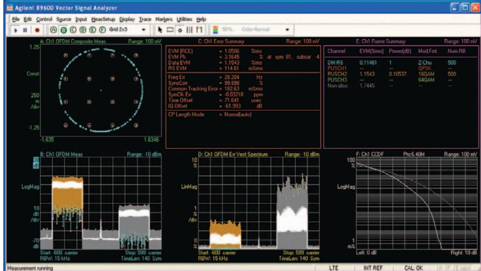
Figure 14. Analysis of a 16QAM SC-FDMA signal
