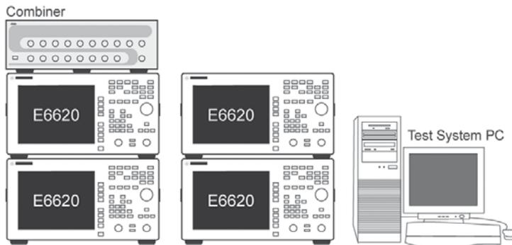
Figure 38. Example of RF-based Anite test system
