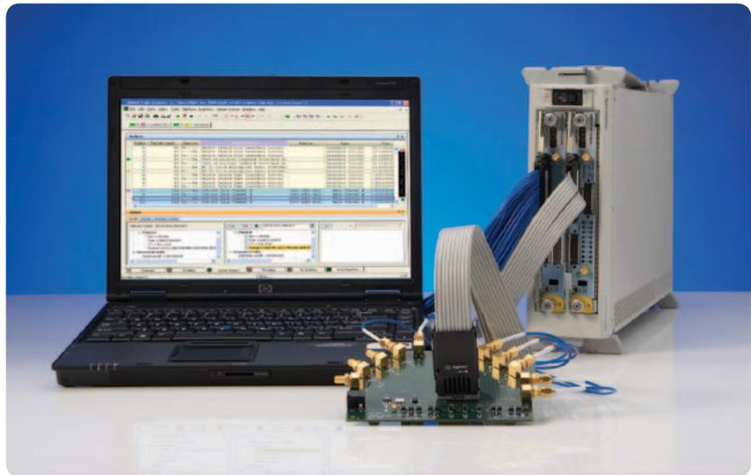
Figure 35. Test platform for access to DigRF v3 and v4 interfaces as well as digital IQ data
