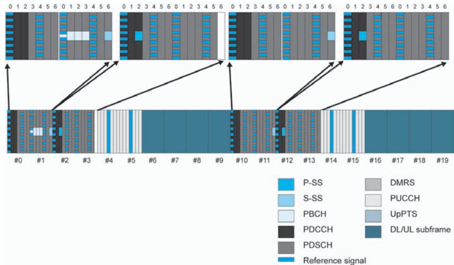
Figure 29. Example of LTE TDD 10 ms switch periodicity mapping
