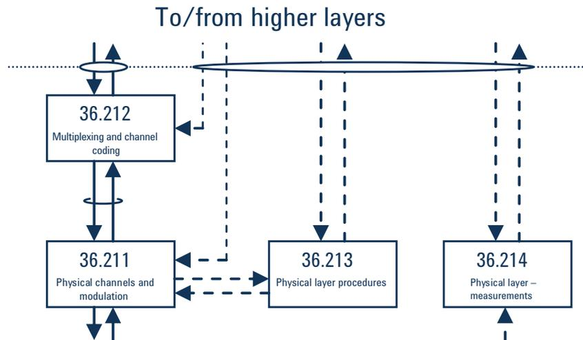
Figure 20. Relation between physical layer specifications (36.201 [11] Figure 2)
