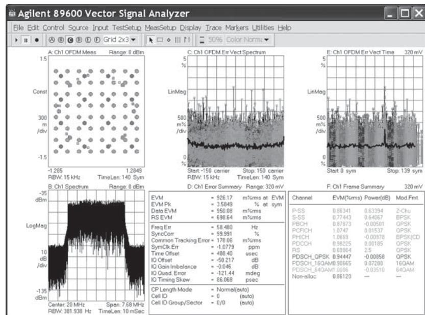
Figure 36. Analysis of digitally demodulated 5 MHz LTE downlink signal using VSA software
