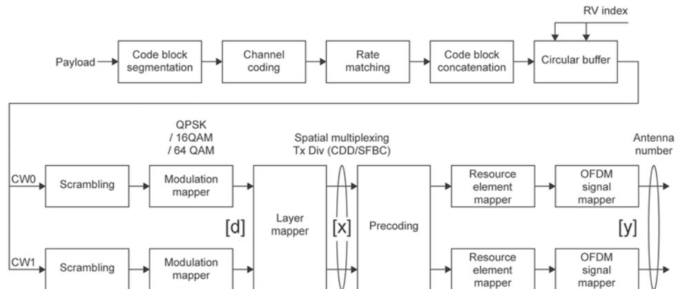
Figure 17. Signal processing for transmit diversity and spatial multiplexing (MIMO) (adapted from 36.211 [10] Figure 6.3-1)
