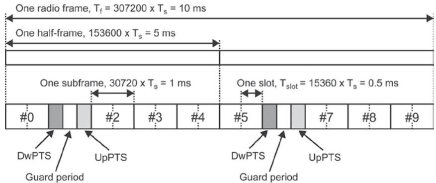
Figure 22. LTE frame structure type 2 for 5 ms switch-point periodicity (based on 36.211 [10] Figure 4.2-1)
