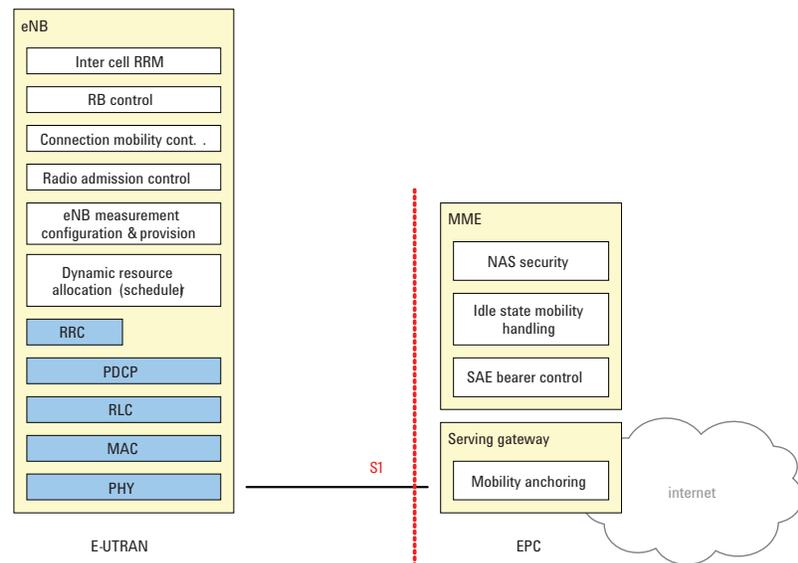
Figure 5. Functional split between E-UTRAN and EPC (36.300 [4] Figure 4.1)
