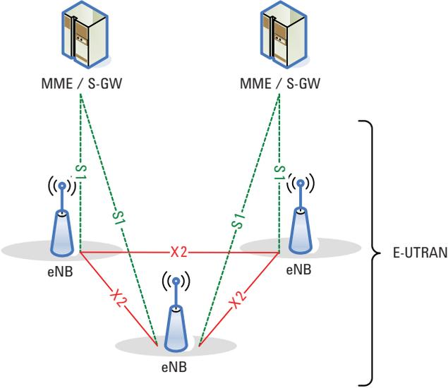
Figure 4. LTE architecture with E-UTRAN (36.300 [4] Figure 4)
