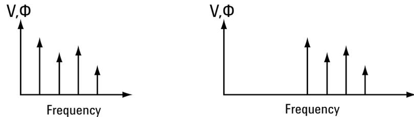
Figure 11. Baseband and frequency shifted DFT representations of an SC-FDMA symbol
