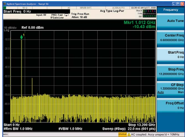
Figure 5b. The MXA only takes 22 ms for a full span of 13.2 GHz sweep (RBW=VBW=1 MHz).
