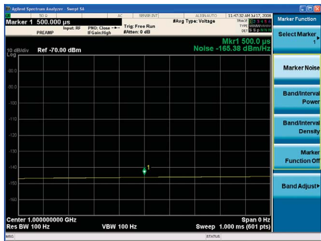
Figure 6b. An MXA shows -165.38 dBm DANL normalized to RBW of 1 Hz, with the preamplifier on.
