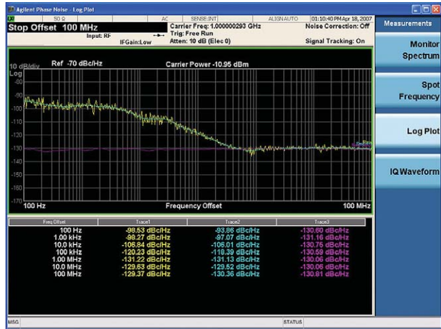
Figure 11b. Phase noise log plot obtained with N9068A phase noise measurement application in an MXA—much faster and easier to use than the 85671A.
