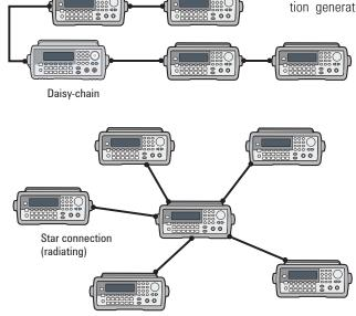
FIGURE 1. Examples of how to connect the time bases of multiple generators, using the star and daisy chain configurations.
