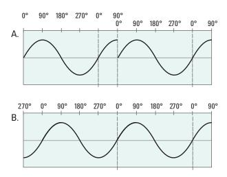
FIGURE 2. A) Use the phase adjust to cause a one-time shift or "bump" in the signal.
