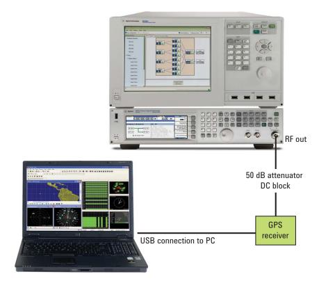
Figure 5. Typical GPS receiver test setup.
