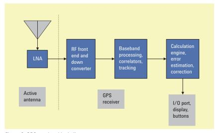
Figure 2. GPS receiver block diagram.
