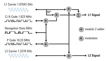
Figure 1. GPS signal structure.
