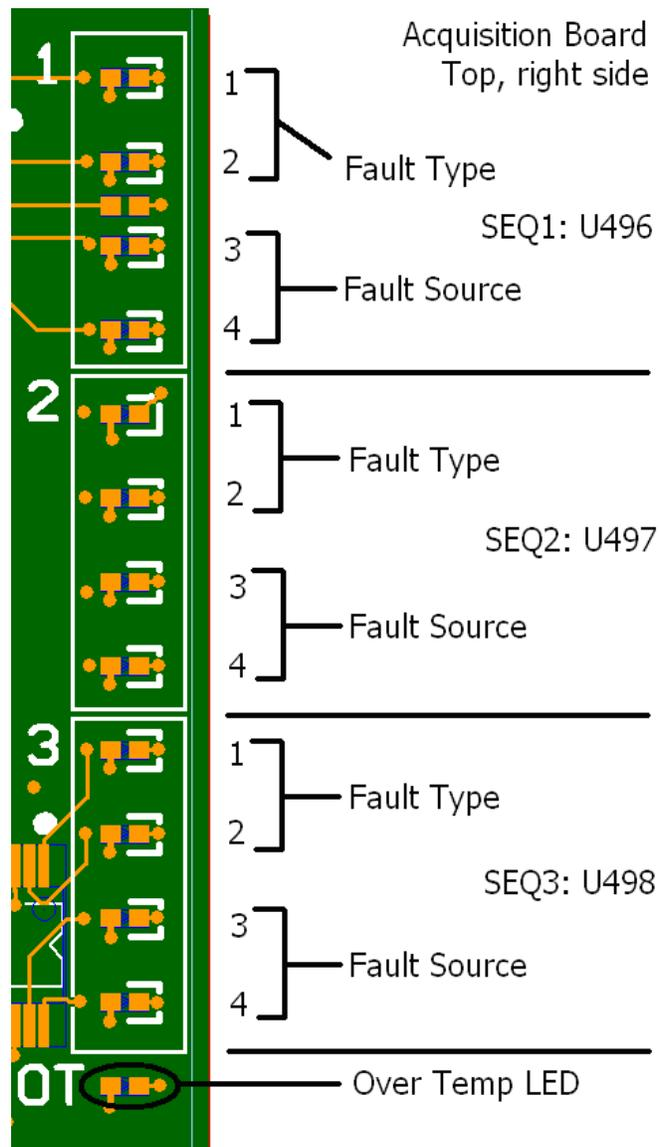
By looking at the pattern of LEDs illuminated after a power failure, you can determine the cause of the fault. However, in most cases, only assembly level repair is required which greatly simplifies decoding these LEDs. An in-depth discussion of these LEDs will first be presented so you understand how they operate and then the assembly level repair procedures will be discussed.
