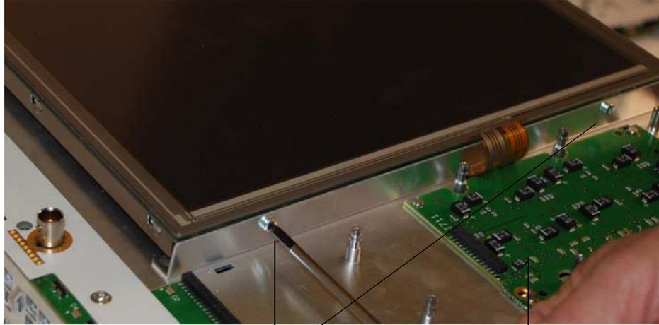
**Remove these two screws and the two on the other side of the touchscreen**
