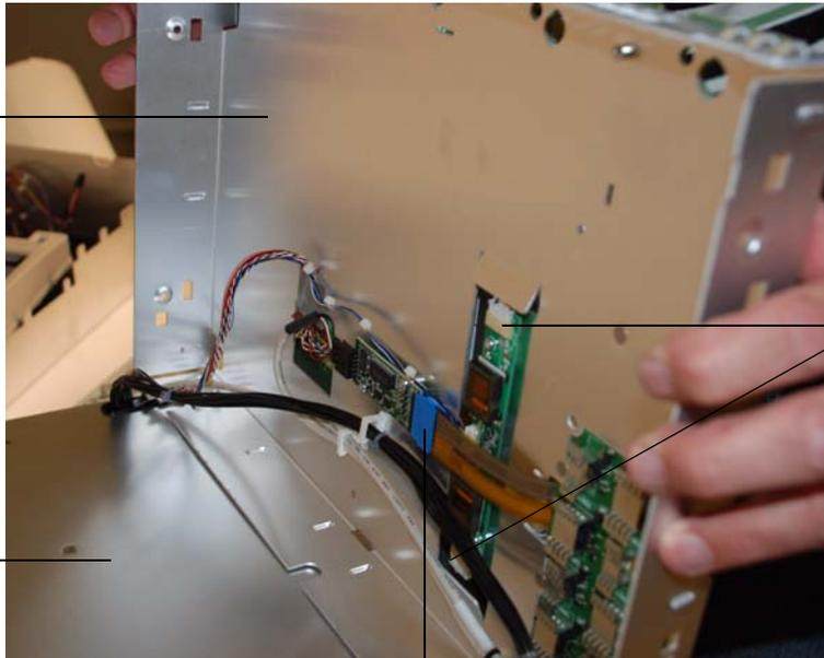
Remove these two display cables (white connectors) from the inverter board because they are connected to the touchscreen display
