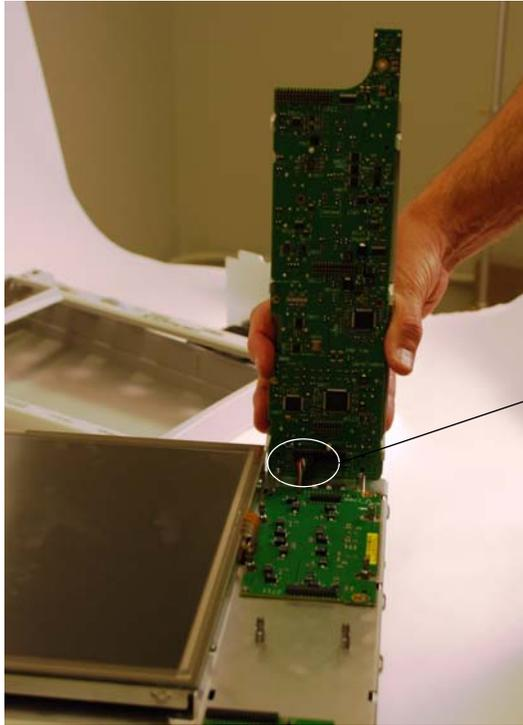
This is where the cable is connected to the front panel keyboard
