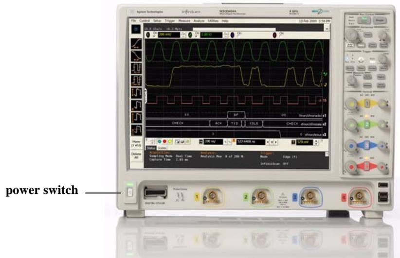
**Turning on the Oscilloscope**
