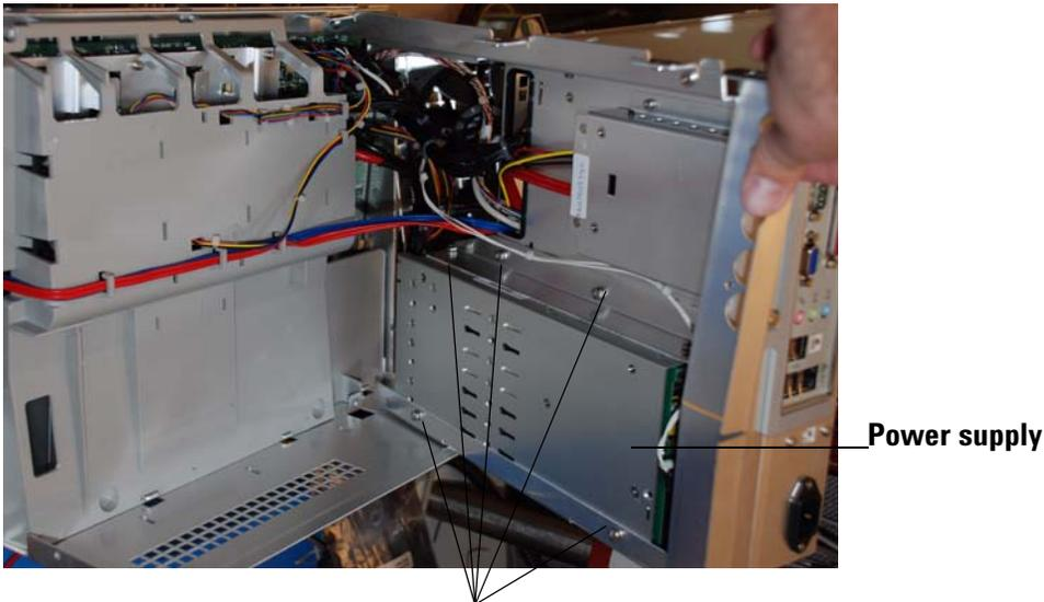
**Remove these screws to lift the power supply and its encasement out.**
