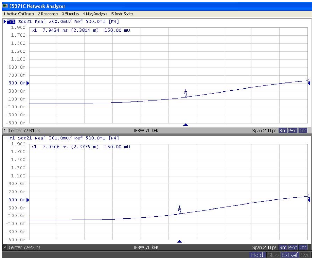
Figure 5.8.6 Inter-Pair Skew Measurement Result Example
