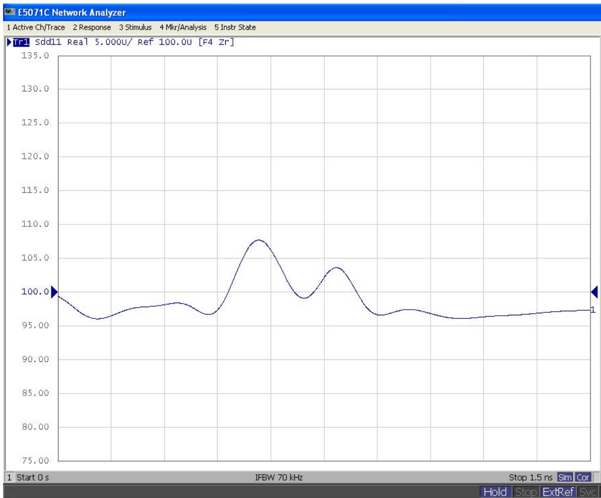
Figure 5.6.3 Impedance Measurement Result Example
