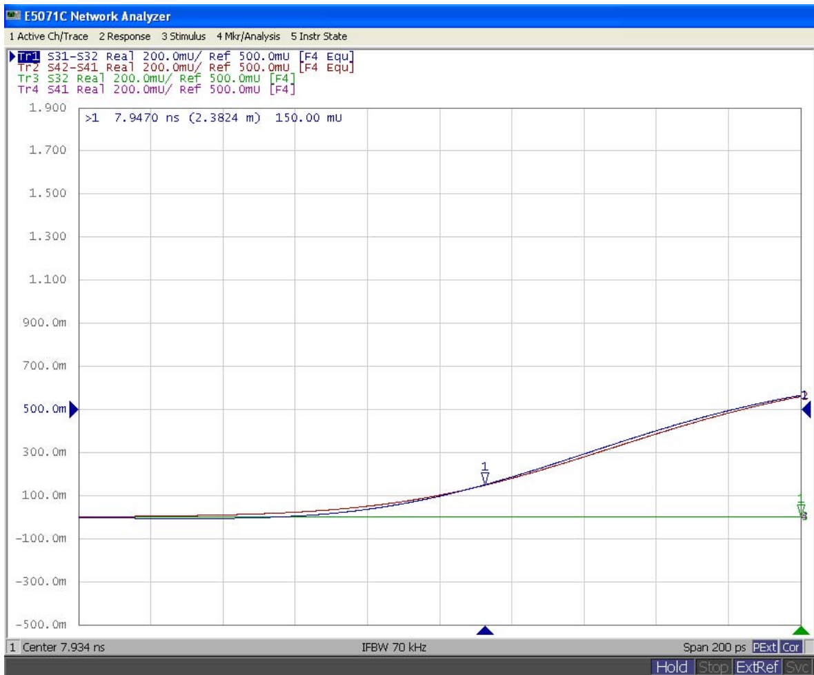
Figure 5.7.6 Intra-Pair Skew Measurement Result Example
