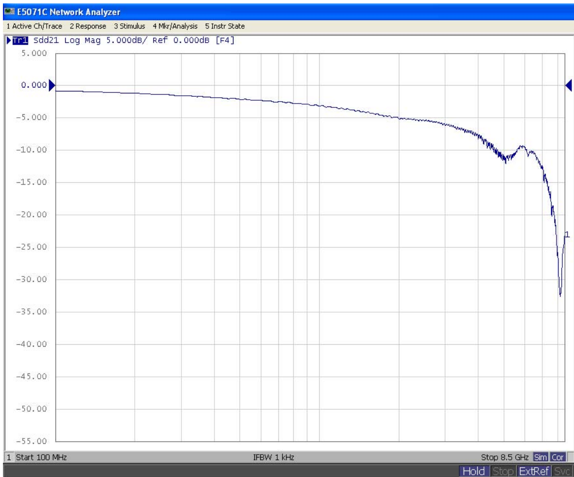
Figure 5.2.2 Insertion Loss Measurement Result Example
