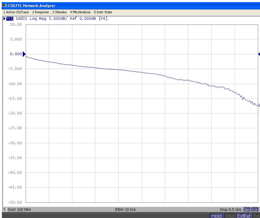
Figure 5-12 Insertion Loss Measurement Result Example
