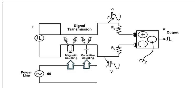
Figure 6-2. Differential active probe provides much higher common mode rejection ratio effectively eliminating common mode noise current.
