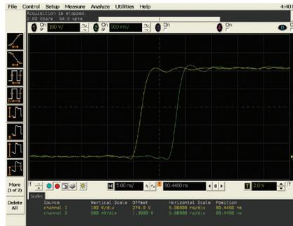
Figure 2-3. Reduced probe loading with short ground lead
