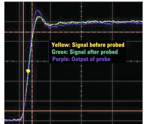
Keysight N2796A 2-GHz active probe with 1.8-cm ground lead
