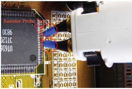
This probe’s damped accessories give a flexible use model that maintains low input capacitance and inductance and flat frequency response through its specified bandwidth. The InfiniiMode N2750A Series, 1156A-58A Series and InfiniiMax Series probes use this damped accessory technology for optimum, but flexible performance.
