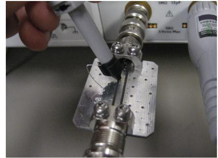
In Figure 2-3, the same signal ground is probed with a short spring-loaded ground lead. The ringing on the probed signal (purple trace) went away with the shorter ground lead.
