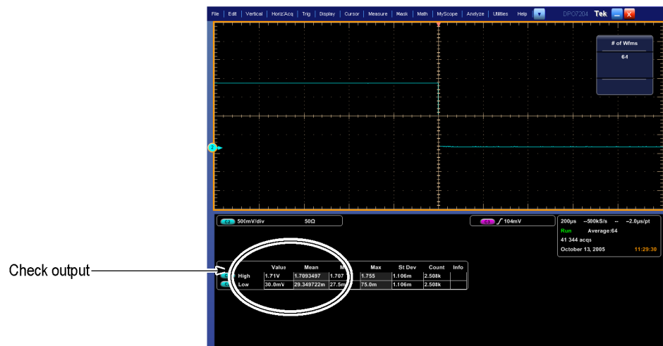
Figure 2-29: Measurement of trigger out limits
