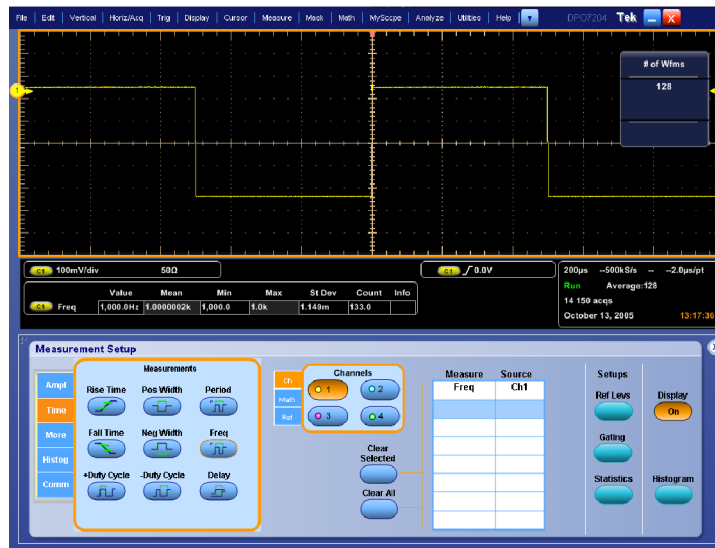
Figure 2-31: Measurement of probe compensator frequency
