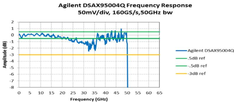
Figure 7. Keysight DSAX95004Q frequency response plot.
