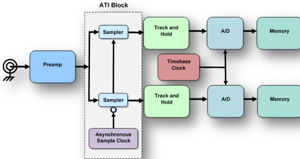
Figure 10. Asynchronous time interleave circuit.
