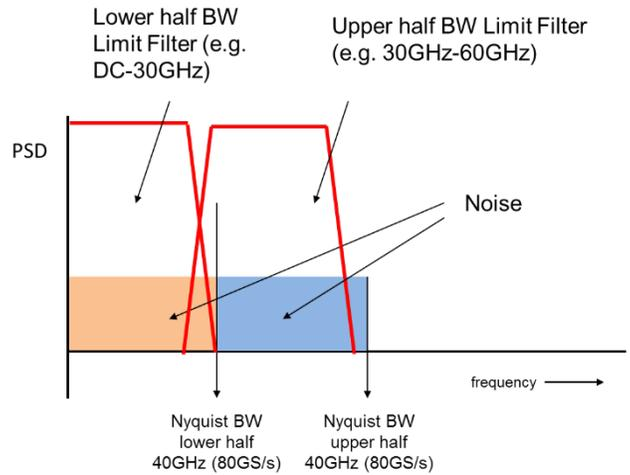
Figure 8. Noise Power Spectral Density across Nyquist bandwidth.
