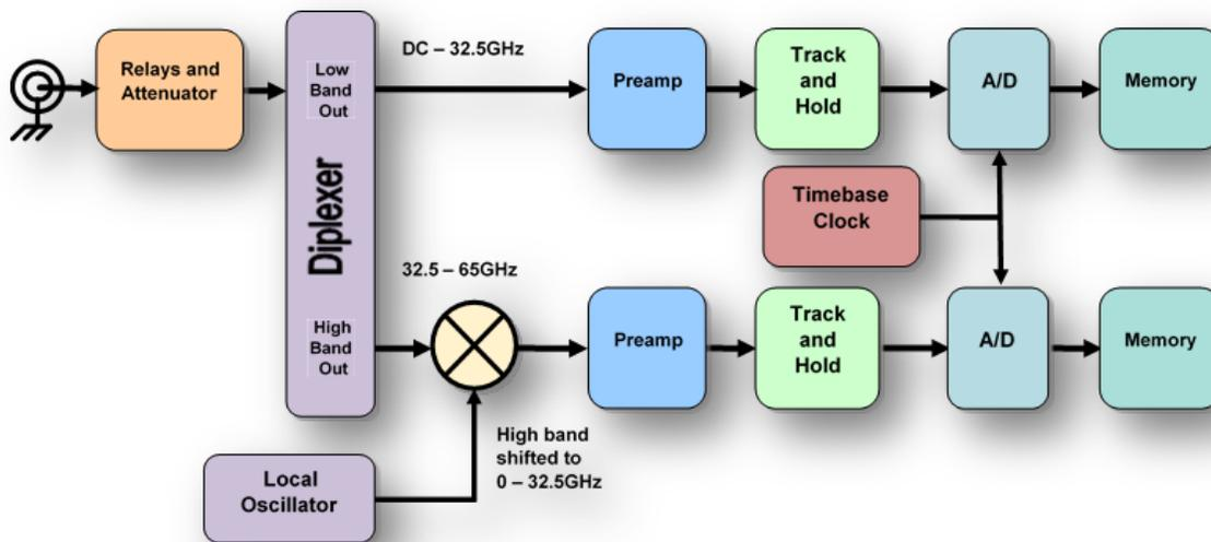
Figure 5. Example of a mixer-based acquisition channel.
