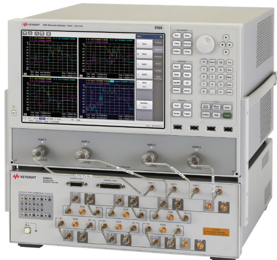
Figure 14. Multiport configuration with E5080A and E5092A
