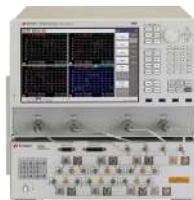
E5080A ENA with E5092A configurable multiport test set
